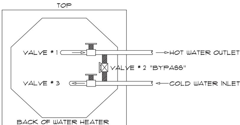
**Diagram # 2: winterizing procedure & the addition of potable non-toxic antifreeze**
